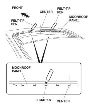
Locate the panel folding line on the right side of the moonroof opening. Measure 87 mm to the front of the vehicle, and make a mark on the roof. Repeat on the other side of the moonroof opening.
