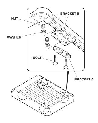
11. Position the roof basket on the roof rack, with the flap from frame A facing forward. Attach the basket to the cross bars by sliding bracket A around the crossbar and tightening the nuts. Tighten the nuts evenly.
