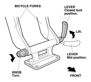
NOTE: After installing the bicycle on the bicycle attachment, secondary strapping on both sides are needed to secure the bicycle to the vehicle bed.
