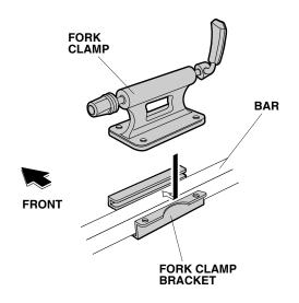
6. Using a torx wrench provided, secure the fork clamp to the bar with two bolts, two 6 mm washers, and the fork clamp bracket.
