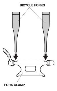
Lift the lever from the mid position to the closed lock position and while holding the lever on the fork clamp, turn the knob on the fork clamps to tension the bicycle forks.
