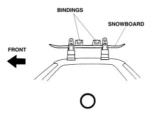
11. If the bindings cannot be positioned between the front and the rear attachments, install the snowboard astride the rear attachment as shown.
