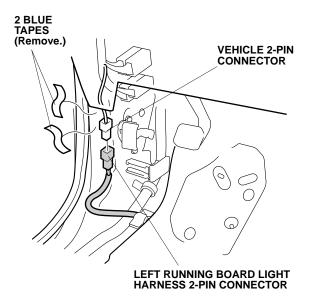
25. Plug the left running board light harness 2-pin connector into the vehicle 2-pin connector.
