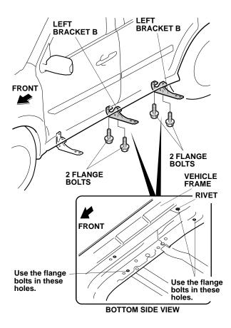
12. Position the left running board on the left bracket A and the two left brackets B. Install the left running board with the six flange nuts. Do not tighten the flange nuts yet.
