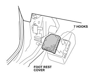
6. Remove the foot rest (two flange nuts).
