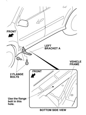
3. Position the left two brackets B at the respective installation positions of the vehicle frame. Install the two left brackets B on the vehicle frame with the two flange bolts for each. Do not tighten the flange bolts yet. Make sure the flange bolts are installed in the correct positions.
