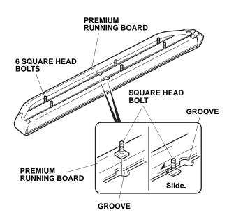
5. Position the premium running board on the left bracket A and two left brackets B. Install the premium running board with the six flange nuts. Do not tighten the flange nuts yet.
