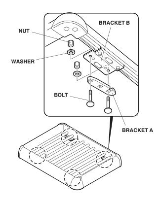
11. Position the luggage basket on the roof rack, with the flap from frame A facing forward. Attach the basket to the cross bars by sliding bracket A around the crossbar and tightening the nuts. Tighten the nuts evenly.
