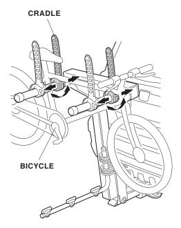
When loading two bicycles, alternate the direction of the bicycles.
