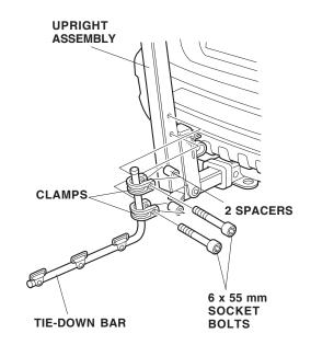
6. Turn the tie-down bar 90° in the direction shown. This is the stored position.
