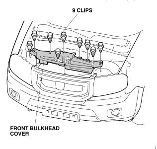
2. Remove the front bumper (nine clips, four bolts, and four self-tapping screws). Have an assistant help you when removing and installing the front bumper. If the vehicle is equipped with the foglight or the front corner sensors, unplug the connectors. Place the front bumper on a blanket after removal.
