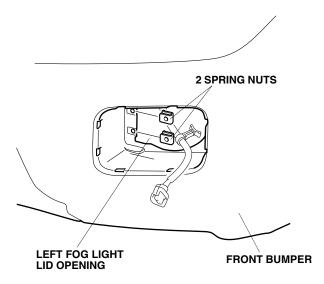
20. Plug the fog light harness 2-pin connector to the left fog light.
