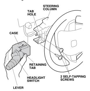
32. Install the new headlight switch on the steering column using the two self-tapping screws. Hold the case by hand, then install the new headlight switch to the steering column. Do not push the lever when installing the case. Push the case and set the retaining tab to the tab hole securely.
