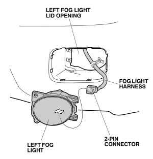
21. Insert the two hooks of the left fog light into the front bumper, and install the left fog light on the front bumper with two 5 x 16 mm washer-bolts.
