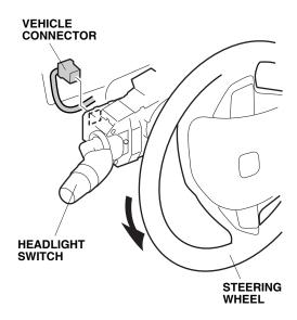
31. Remove the two self-tapping screws from the headlight switch. While pushing the retaining tab, slide the headlight switch, and remove it from the steering column. Do not pull out the lever when removing the case. Do not damage the tab hole of the steering column.
