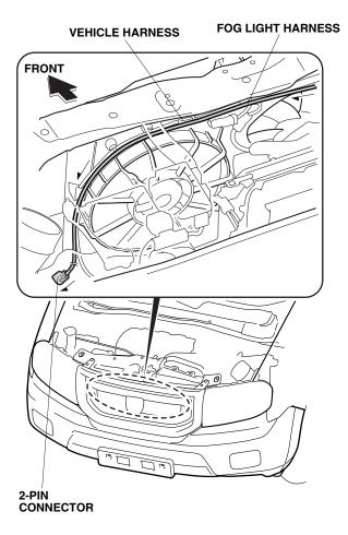
14. Route the fog light harness 2-pin connector (longer position of the harness) to the underside of the vehicle.
