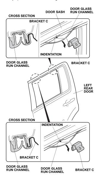
11. Peel the door glass run channel and install two brackets C to the left rear door as shown. Make sure that the brackets are installed in the correct position. Check that the brackets and the door glass run channel is installed on the door sash properly. 12. Peel back approximately 1-1/2 to 2 inches of adhesive backing from each adhesive tape, and tape the ends to the front surface of the left rear door visor with a masking tape.
