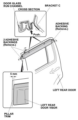
16. Remove the adhesive backings from the left rear door visor.
