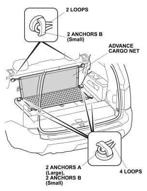
20. Attach six loops on the advance cargo net to two anchors A (Large) and four anchors B (Small) on the second and third row seat back board.
