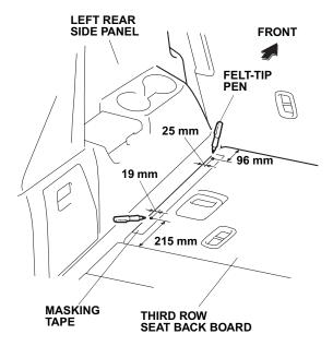
6. While wearing eye protection, drill at the marked locations with a 3 mm drill bit and then with a 5 mm drill bit then drill through the hard board and sheet metal. To prevent damage to the inner vehicle parts, wrap tape around the drill bit 25 mm away from the tip as shown.
