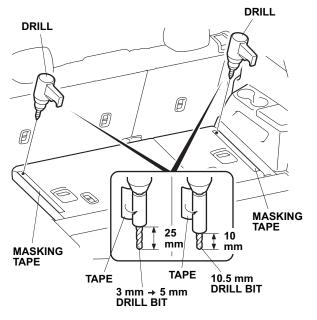
7. Drill at the marked location with a 10.5 mm drill bit. To drill through the hard board only, wrap tape around the drill bit 10 mm away from the tip as shown.
