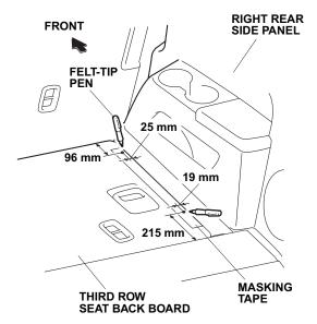
5. Using a felt-tip pen, measure and mark two locations on the masking tape attached in step 3.
