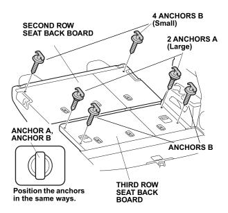
18. Install the four anchors B (Small) on the second and third row seat back board into the holes made in step 8 and 13.
