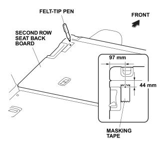
13. While wearing eye protection, drill at the marked locations with a 3 mm drill bit and then with a 5 mm drill bit then drill through the hard board and sheet metal. To prevent damage to the inner vehicle parts, wrap tape around the drill bit 25 mm away from the tip to the root as shown.
