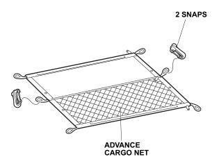
28. Attach four loops on the advance cargo net to two hooks and two anchors B (Small) on the third row seat back board.
