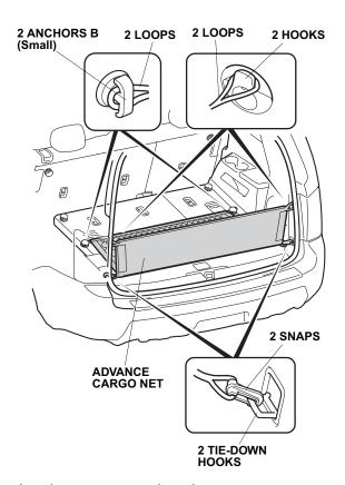
29. Attach two snaps on the advance cargo net to two tie-down hooks.
