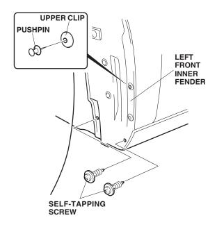
Using a pushpin, make a small hole through the center of the upper clip.
