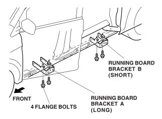
7. Temporarily secure the running board brackets C to the running board bracket A (long) and B (short) with four flange bolts and four flange nuts as shown.
