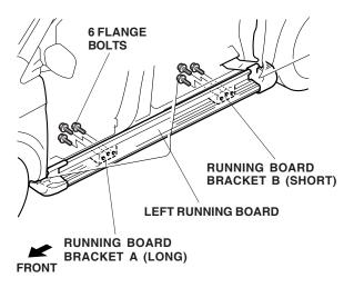
20. Loosen the remaining eight flange bolts securing the running board bracket A (long) and B (short).
