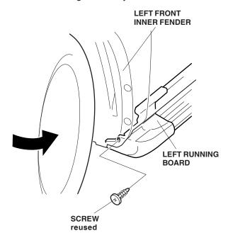
18. Remove the screw securing the left running board.
