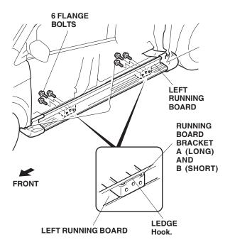
14. Tighten the 10 flange bolts and four flange nuts temporarily secured in steps 6 thru 8.
