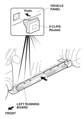
13. Hook the left running board to the ledge on the running board bracket A (long) and B (short) as shown. Install the left running board with six flange bolts. Torque the flange bolts to 27 N·m (20 lb-ft).
