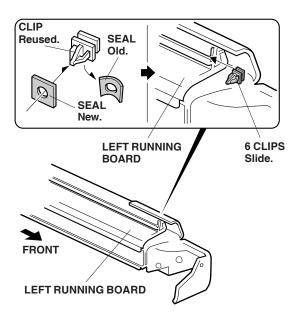
12. Hold the running board up and fit all the clips into the holes in the body, then push on the top of the running board until the clips snap into place.
