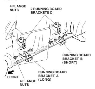
8. Temporarily secure the running board bracket C to the vehicle with two flange bolts at the indicated holes as shown.
