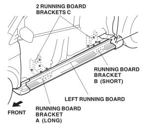
15. Secure the left running board with the screw you removed in step 2 to the left front inner fender as shown.
