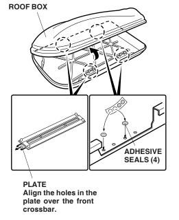
3. Attach an adhesive seal over the unused rear mounting holes along the bottom of the roof box. The seal will help prevent water from entering the roof box. Remove the roof box from the vehicle.
