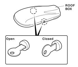
**Locking**: Press down on the lid. There should be an audible click. Be sure the lid is latched by attempting to lift the lid. Turn the key clockwise to lock the roof box. Remove the key while not in use. Be sure the straps are not outside of the roof box.
