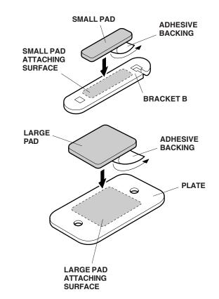
Using isopropyl alcohol on a shop towel, clean the four plates where the large pads will attach.
