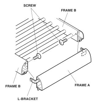
6. Attach the remaining frame A to frame B in the same way.
