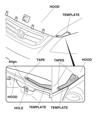
6. Using an alcohol swab, clean the area where the left bracket B will mount. Remove the adhesive backing from the left bracket B, and align it to the template secured in step 5.
