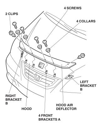
10. Insert the large end of the template between the hood and the hood air deflector molding, as shown, to unfold the molding.
