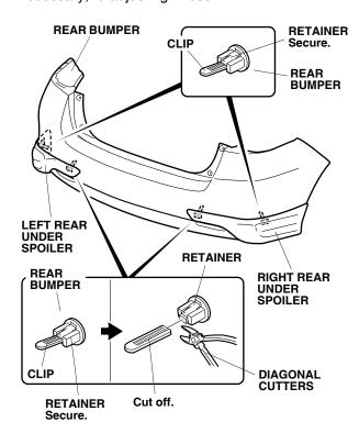
29. Using diagonal cutters, cut off and remove the excess clip end.
