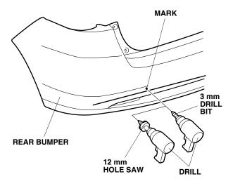
5. On the inside of the rear bumper on the left side, tape the template to the inside edge in the area shown.
