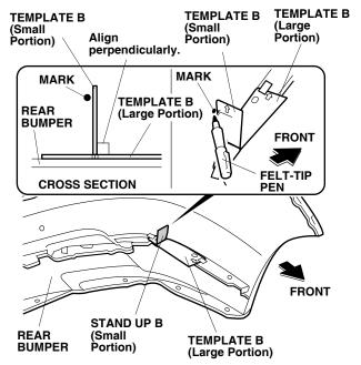
12. Using a pushpin, pierce the bumper at the mark you made on the bumper.
