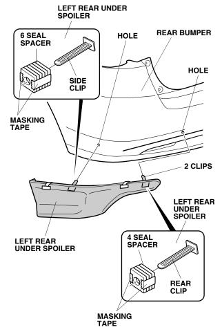
20. Install one six seal spacer over the side clip, install the four seal spacer over the rear clip, and install the left under spoiler to the bumper.
