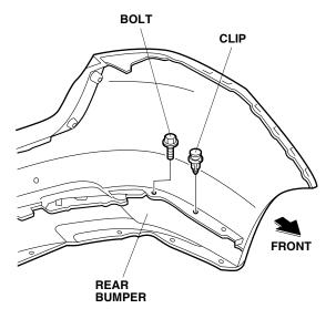
Tape template B (large portion) to the bumpers and align the hole in the template with bolt and clip hole.
