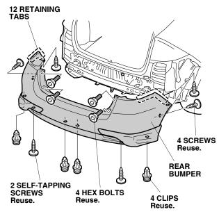
31. Tighten the four self-tapping screws and the two flange bolts you loosely installed secured in step 23.
