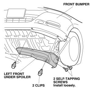
10. Loosely install two self-tapping screws to secure the left front under spoiler.
