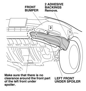
12. Using the palm of your hand, firmly press the left front under spoiler against the front bumper. Make sure that there is no clearance around the front part of the left front under spoiler.
