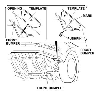
3. Remove the template from the front bumper, and reinstall the air spoiler.
