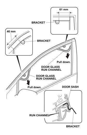
3. Install two brackets between the door sash and the run channel at the measurements shown. Seat the door glass run channel properly around the brackets.
