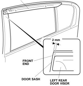
19. While holding the door visor up firmly, remove the adhesive backing. Use your finger to push up each bracket so there is no gap between the brackets and the door sash.
