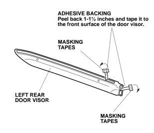
17. Align the clip holes in the visor with the bracket holes, and install two clips. There should be no clearance between the brackets and the door sash.
