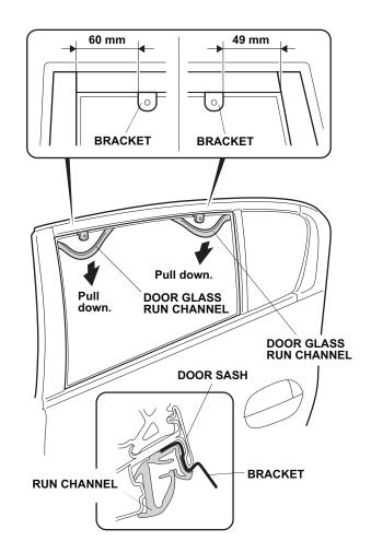
13. Install two brackets between the door sash and the run channel at the measurments shown. Seat the run channel properly around the brackets.
