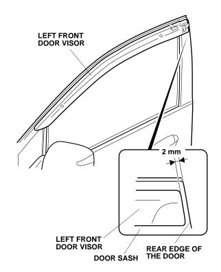
9. While holding the door visor up firmly and back against the rear edge, remove the adhesive backing. Use your finger to push up each bracket so there is no gap between the brackets and the door sash.
