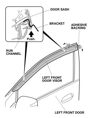
10. Using a soft towel, press and hold the door visor against the door sash for 30 seconds.
