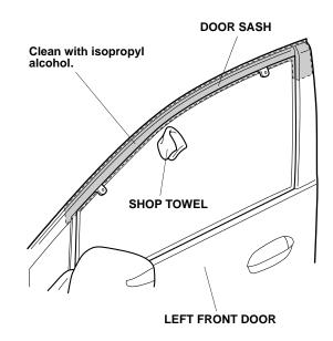
5. Remove the adhesive backing from the seal, and attach it to the door sash.
