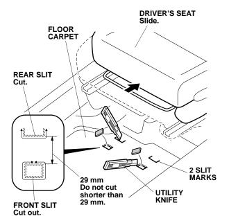
3. Locate the two front reccesses in the floor carpet Using a utility knife, cut out each front reccess. Make sure the distance between the slit and the cutout is not les than 29 mm.
