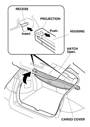
2. Insert the left end of the cargo cover into the recess on the left rear side trim panel. Push the end further into the recess, hold it in that position, then insert the right end into the recess on the right side trim panel.
