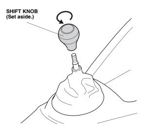
2. Install the new shift knob by turning it clockwise. Turn the knob until the orientation of the shift pattern is correct. The knob should turn 10 to 14 times.
