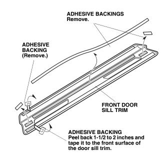
4. Clean the surface where the front door sill trim will be installed using an alcohol swab.
