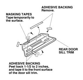
11. Clean the surface where the rear door sill trim will be installed using an alcohol swab.
