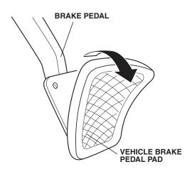
8. Using isopropyl alcohol on a shop towel, clean the brake pedal. Allow the alcohol to dry.
