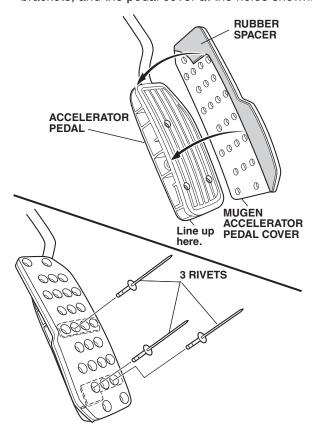
6. Place one spacer on each rivet. Using the rivet tool, compress each rivet while holding the spacer tight against the pedal. Remove the spacers.
