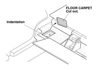
5. Fold back the carpet, and install one tie-down using the attached bolt.
