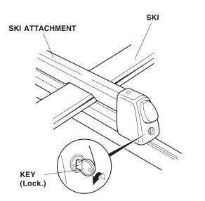
5. With the skis attached, rock the attachment in all directions to make sure it is installed securely. Adjust as necessary.
