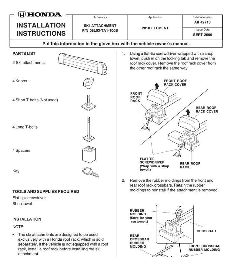
• The ski attachments may be installed either with both on the driver's side or with both on the passenger's side.
