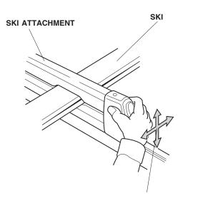
Rock the ski attachment in all directions to make sure it is installed securely.
