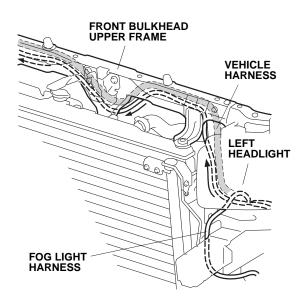
22. Continue routing the fog light harness 2-pin connector forward, then down to the bottom of the front side frame along the outside of the right bulkhead side stay.
