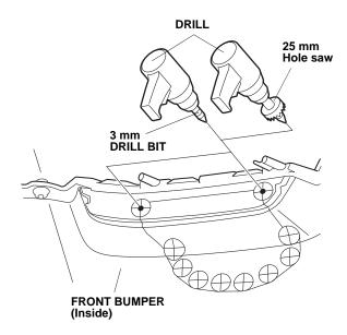
8. On the outer surface of the bumper, drill the remaining eight pierced marks to 25 mm. While wearing eye protection, drill with a 3 mm drill bit, and then finish with a 25 mm hole saw.
