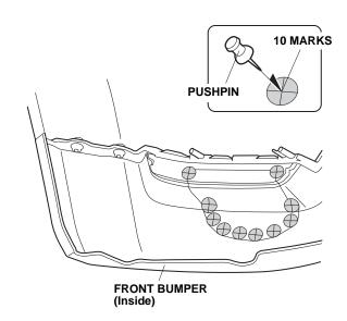
6. Attach masking tape to the outer surface of the bumper in the areas shown.
