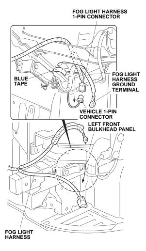
17. Locate the 1-pin connector blue-taped to the vehicle harness and remove the blue tape to free the 1-pin connector. Plug the 1-pin connector you just freed into the fog light harness 1-pin connector.
