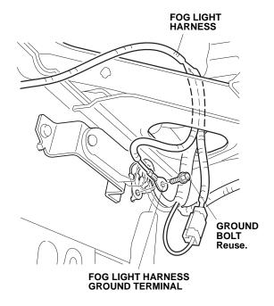
19. Secure the fog light harness 1-pin connector to the vehicle harness with one wire tie. Do not secure the connector to the SRS harness.
