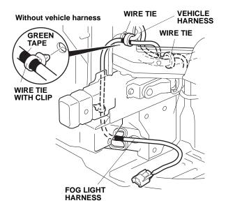
28. Secure the fog light harness to the vehicle harness with one wire tie.
