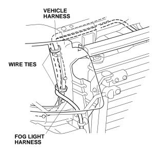
26. Secure the fog light harness to the vehicle harness with seven wire ties in the areas shown.
