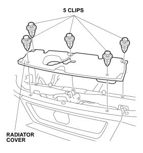
4. With the help of an assistant, remove the front bumper (five clips, four stepped bolts, and four self-tapping screws). Place the front bumper on a blanket to prevent damage.
