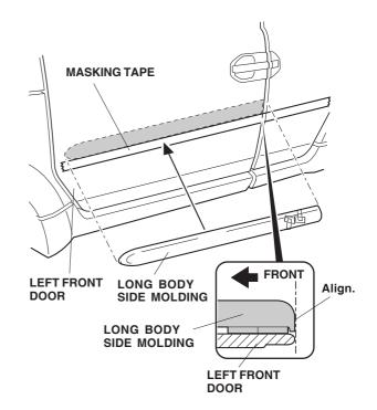
5. While applying light pressure on the body, carefully remove the adhesive backings from the long body side molding.
