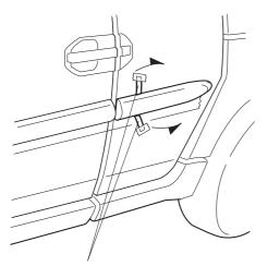
ADHESIVE BACKINGS While holding pressure on the molding, slowly and carefully remove the adhesive backing. After removing all adhesive backings, hold the molding firmly against the door with the palm of your hand.
