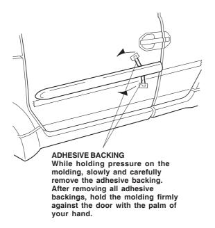
6. Using a hard rubber roller, roll the long body side molding from one end to the other.
