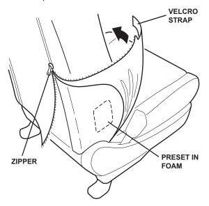
4. Using a utility knife, cut out the foam preset to expose the armrest bracket.
