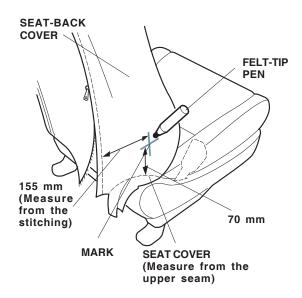
6. Using a utility knife, make two 65 mm (2 1/2 in.) cuts in the seat-back cover to expose the seat base.
