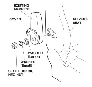
Remove the hex nut, small washer, and large washer that secures the existing armrest, and remove the armrest.
