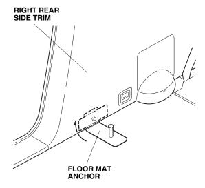
5. Align the floor mat anchor with the hole in the right rear side trim and install the washer-screw. Tighten the washer-screw.
