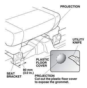
2. Install a front floor mat anchor to each of the three grommets using one self-tapping screw for each floor mat anchor.
