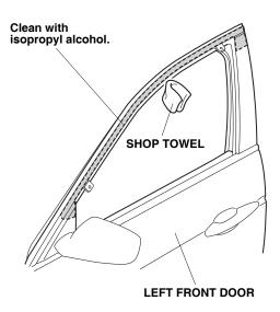
Peel back approximately 25-35 mm (1-1.5 inches) of adhesive backing from each adhesive tape, and tape the ends to the front surface of the left front door visor.
