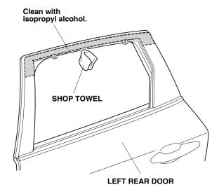
14. Peel back approximately 25-35 mm (1-1.5 inches) of adhesive backing from each adhesive tape, and tape the ends to the front surface of the left rear door visor.
