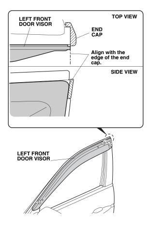
8. While holding the door visor up firmly, remove the adhesive backing in the order shown. Use your finger to push up each bracket so there is no gap between the brackets and the door sash.
