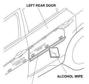
ATTACHING POSITION (Clean using an alcohol wipe.)
