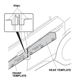
7. Using two alcohol wipes, clean the door surfaces below the templates where the body side moldings will attach. Allow the alcohol to dry.
