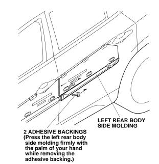
15. Using the rubber roller, apply firm pressure while rolling to set the adhesive. Apply firm pressure especially at the ends.
