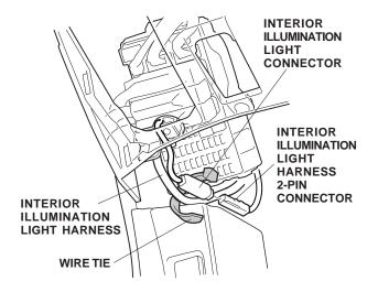
illumination light harness using a wire tie. If the vehicle is equipped with a instrument panel pocket, continue with step 48; otherwise, go to step 51.
