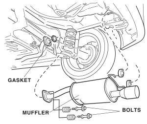
4. Torque the bolts to 22 N⋅m (16 lb-ft), alternating from side to side.
