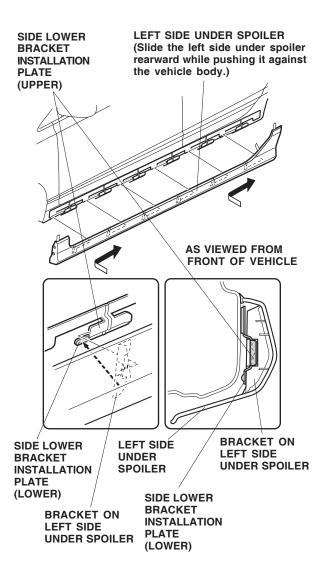
20. Check that all six brackets of the left side under spoiler are set in the side lower bracket installation plates. Visually check that there is no excessive gap between the left under spoiler and the vehicle. If an excessive gap is found, repeat step 19. 21. Fit the under bracket to the side under spoiler and mark the under coat.
