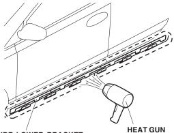
SIDE LOWER BRACKET (Warm up the side lower bracket when the ambient temperature is below 60°F [15°C].)
