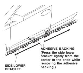
When the ambient temperature is below 60°F (15°C), warm up the entire side lower bracket to 60°F (15°C) or above before attaching it to the vehicle body.
