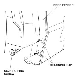
18. Using a self-tapping screw, pierce a hole through the center of the inner fender retaining clips.
