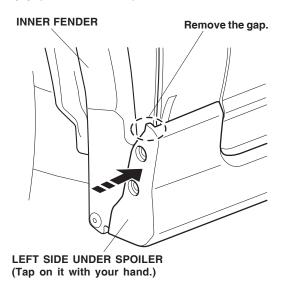
25. Loosely install the front self-tapping screws in the holes in the left side under spoiler at the wheel arch.
