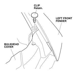
3. Install one new clip with a snap-screw into the hole where you removed the clip, and tighten the snap-screw.
