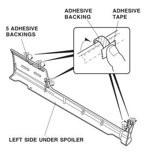
22. Check the position of the under spoiler attachments by looking down at them from the top. While pushing the under spoiler against the vehicle body with both hands, slide the left side under spoiler rearward. Make sure the location of the side lower bracket installation plates (upper and lower) attach to the brackets on the left side under spoiler.
