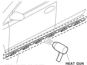
SIDE LOWER BRACKET (Warm up the side lower bracket when the ambient temperature is below 60°F (15°C).)
