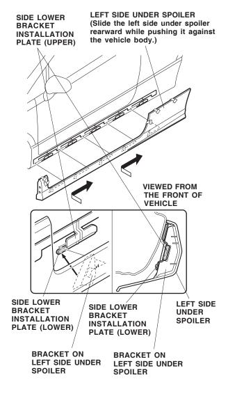
23. Check that all six brackets on the left side under spoiler are set in the side lower bracket installation plates. Visually check that there is no excessive gap between the left under spoiler and the vehicle. If an excessive gap is found, repeat step 22.
