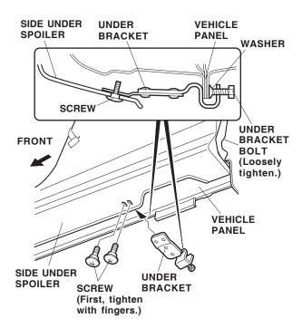
Position the under bracket on the side under spoiler, and loosely install the two screws. Tighten the under bracket bolt, but don't tighten it completely yet. 31. Align the rear top edge of the left side under spoiler with the edge of the radius of the vehicle panel as shown. Remove the five adhesive tapes from the left side under spoiler. Press firmly on the side under spoiler.
