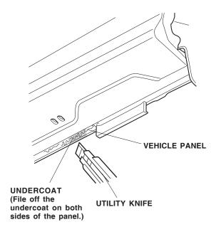
Apply touch-up paint to the vehicle panel in the area where you filed off the undercoat. Do not install the under bracket until the touch-up paint dries. 27. Gently tap on the left side under spoiler to remove any gap between the spoiler and the wheel arch.
