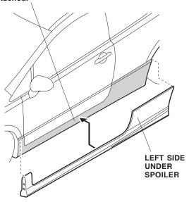
2. Using a tape measure and felt-tip pen, measure and mark the body as shown.
