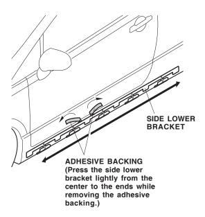
When the ambient temperature is below 60°F (15°C), warm up the entire side lower bracket to 60°F (15°C) or above before attaching it to the vehicle body.
