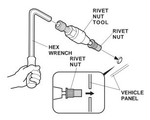
7. While holding the tool with the hex wrench, rotate the 27 mm wrench clockwise and install the rivet nut on the vehicle panel.
