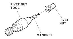
6. Insert the rivet nut into the hole in the vehicle panel.
