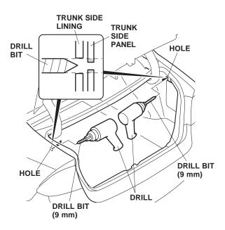
4. Install two rivet nuts into the 9 mm holes you enlarged in step 3.
