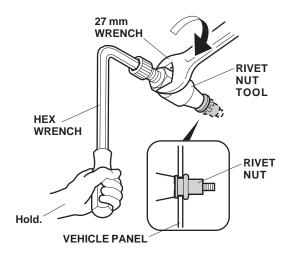
8. Remove the tool from the rivet nut by turning the hex wrench counterclockwise.
