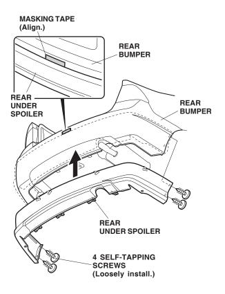
While applying pressure to the rear under spoiler, use a felt-tip pen to mark the rear bumper along each hole in the bracket on the rear under spoiler.
