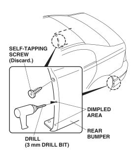
3. Remove and discard the two self-tapping screws from the fenderwell area of the rear bumper.
