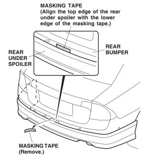
14. While applying pressure on the rear under spoiler, carefully remove the adhesive backings in the sequence shown. After removing, hold the rear under spoiler firmly against the rear bumper with the palm of your hand for 30 seconds.
