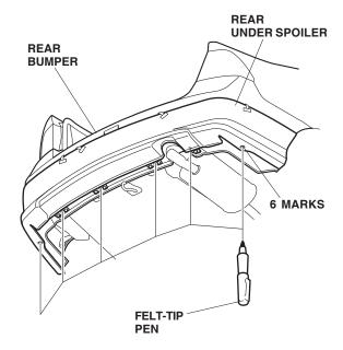
NOTE: If a gap is visible between the rear bumper and under spoiler, remove the under spoiler and confirm the location of the marks with a tape measure. If necessary, create new marks in the proper locations.
