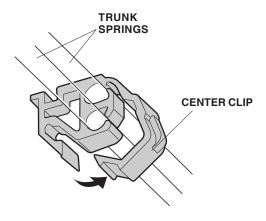
4. With an assistant holding the trunk lid open, remove the old trunk springs from the trunk hinge arms using the special tool. Wear gloves to protect your hands, and pull the special tool slowly and carefully toward you.
