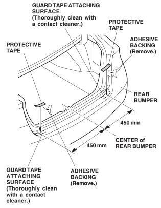
7. Remove the adhesive backing from each of the protective tapes, and attach the tapes to the rear bumper as shown.
