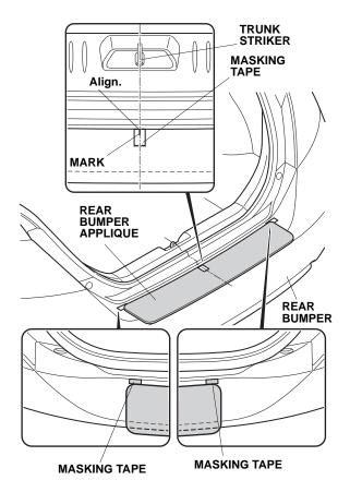
6. Remove the backing shown. Using the applicator with soft sleeve, apply pressure to smooth out the top surface of the rear bumper applique. If you see any air bubbles, gently peel up that section and work out the air bubbles.
