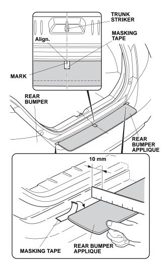
4. Remove the center backing from the rear bumper applique.
