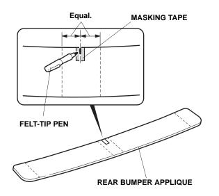
3. Place the rear bumper applique on the rear bumper, then attach masking tape to the rear bumper as shown.
