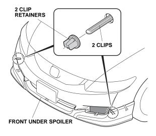
26. With the vehicle on a lift use a pushpin to pierce the front bumper as shown.
