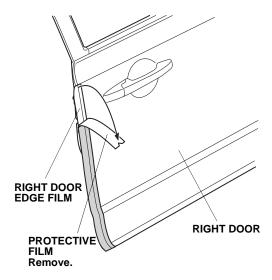
Starting from the middle and working outward, turn back the right door edge film half to the cabin side of the right door as shown. Move your fingers in one direction only.
