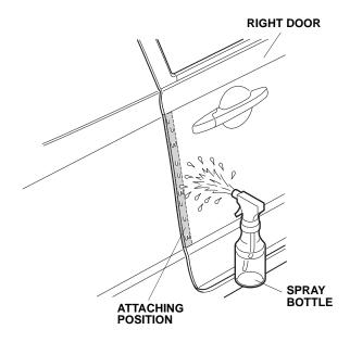
4. Using a spray bottle with 3M protective tape application solution, spray the area where the right door edge film will attach.
