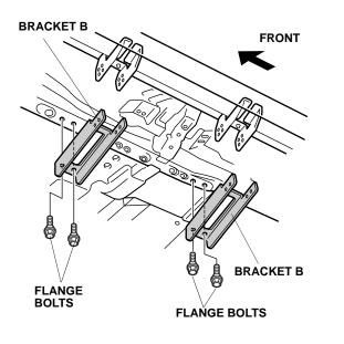
19. Secure brackets A and B using eight flange bolts and eight 8 mm flange nuts.
