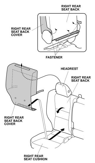
10. Tilt the right rear seat back forward, and tuck the fastener between the seat back and the seat cushion. Secure the three fasteners to the back of the right rear seat back.
