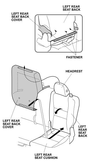
5. Tilt the left rear seat back forward, and tuck the fastener between the seat back and the seat cushion. Secure the three fasteners to the back of the left rear seat back.
