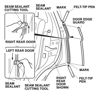
9. Position the cutting edge or the seam sealant cutting tool against the door edge, and trim the seam sealant from mark to mark.
