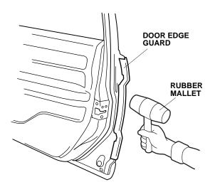
7. Repeat steps 3 thru 6 to install the left front door edge guard.
