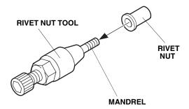
40. Insert the two rivet nuts into the hole in the left trunk side panel and install the hex wrench on the rivet nut tool.
