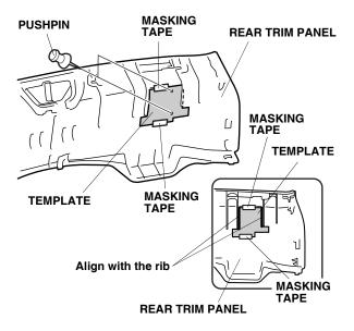
27. While wearing eye protection, drill at the marked points using a drill with 3 mm bit first, finish 6.5 mm bit. Remove any burrs from the edge of the holes using a round file.
