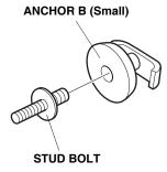
55. Assemble the spacer and the stud bolt on the anchor B (Small).
