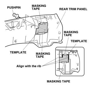
64. Drill at the marked points using a drill with 3 mm bit first, finish 6.5 mm bit. Remove any burrs from the edge of the holes using a round file.
