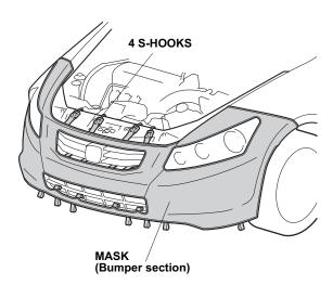
15. Attach the four plastic hooks to the bottom inside edge of the front bumper.
