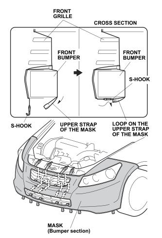
13. Reach under the lower grille and pull the straps out. Attach the four straps to the four hooks on the bottom of the mask. 14. Attach the four S-hooks to the bottom inside edge of the radiator cover.
