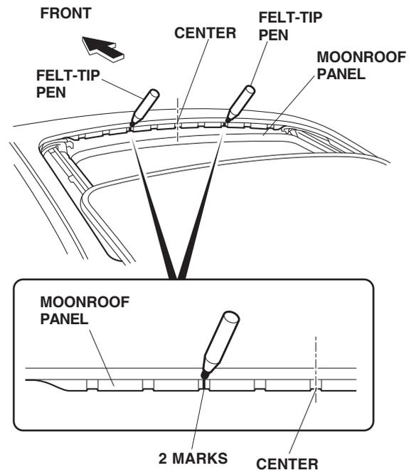
4. Locate the panel folding line on the right side of the moonroof opening. Measure 87 mm to the front of the vehicle, and make a mark on the roof in two places. Repeat on the other side of the moonroof opening.
