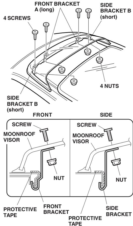
8. While holding the visor in place, install the four screws, four nuts, and four brackets A and B with the end of each bracket hooked to the lip of the moonroof opening. Do not tighten the screws yet.
