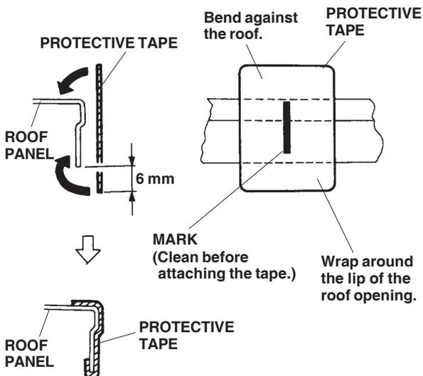
7. Place the two front brackets A into position by sliding them along the lip of the roof opening. Set the moonroof visor on the vehicle roof, in front of the moonroof opening, and adjust its position so the holes in the visor are aligned with the protective tapes.
